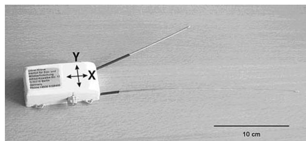
**Fig. 1** Shape and size of the datalogger. The two axes of the acceleration sensors are projected on the device. The long antenna emits VHF signals and the short antenna UHF signals for the download. An address label is attached to increase the recovery of the datalogger
